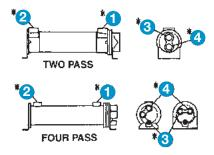
Note baffle location when inserting bundle into shell assembly after cleaning.
