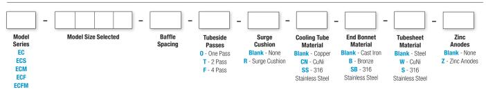
EC = NPT Oil connections; NPT Water connections.
